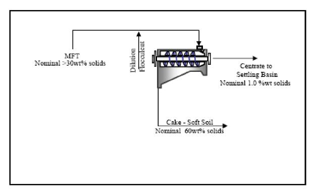
Figure 7. The decanter in the process
