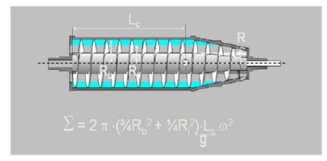
Figure 3. Sigma factor & centrifuge performance
