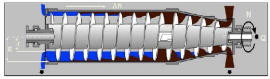
Figure 2. Decanter cross-section
