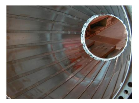
Figure 5. Ribs in the centrifuge bowl
