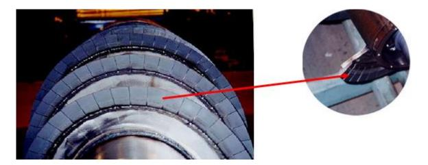
Figure 6. Tiles protect the conveyor flights
