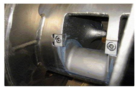
Figure 4. Erosion protection with inserts in the decanter feed zone
